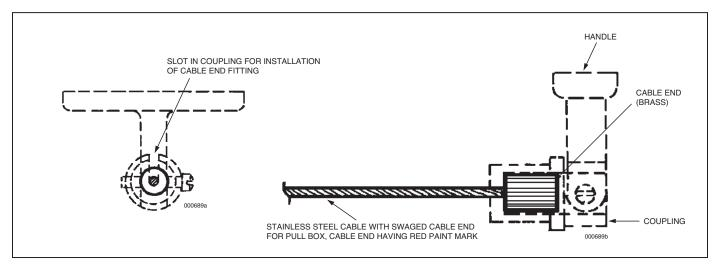
Note: The strength of the end fitting exceeds the breaking point of the cable.
