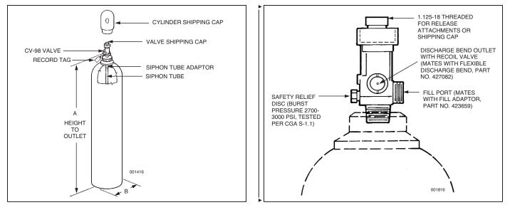
Note: Use Flexible Discharge Bend (Part No. 427082) when attaching valve to supply pipe or manifold.
