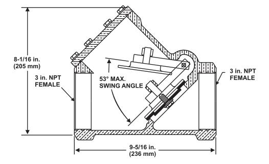
**Note:** The valve must be installed with the arrow pointing in the direction of flow.
