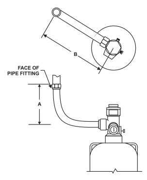
Note: Dimension A and B must be maintained in order to obtain a smooth radius in flexible loop. Hose may require adapter to connect to system piping.
